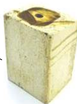
Structure : Bamboo Reinforced Cement ( MgO )
