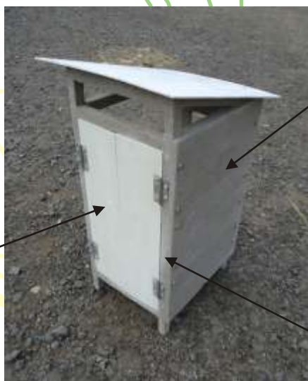
Wall Panels : 4ft x 2 ft Bagas Chip Board +polymer cement composite
